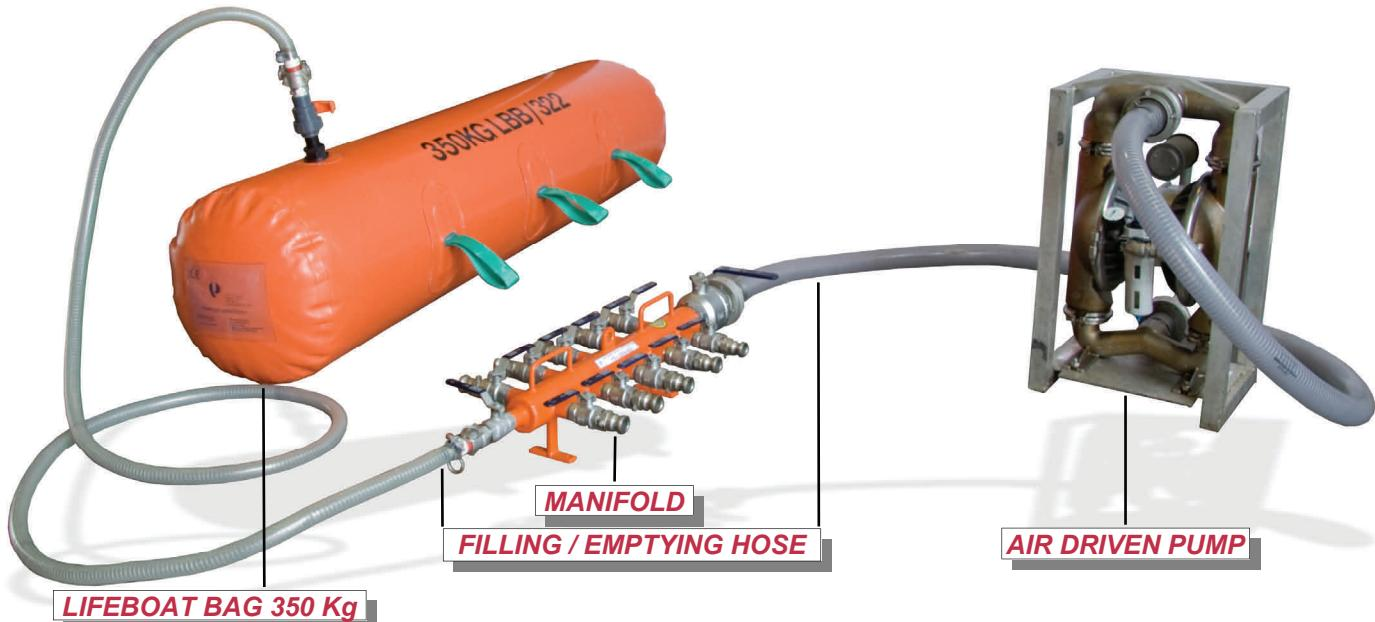
The Lifeboat Bag Test System has a capacity of 6.3 Metric Ton and is a safe and easy to use system for load testing of Lifeboats. The system can also be used for the testing of Crew baskets, gangways or other lifting Equipment. The safety advantage of the system is that it eliminates the need of entering the Lifeboat Capsule during an overload test.
